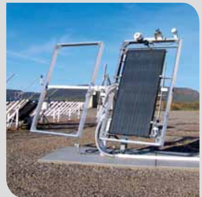
Dual Axis Solar Tracking Rack
