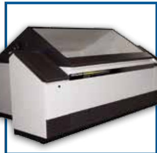
2 Salt Spray Corrosion
